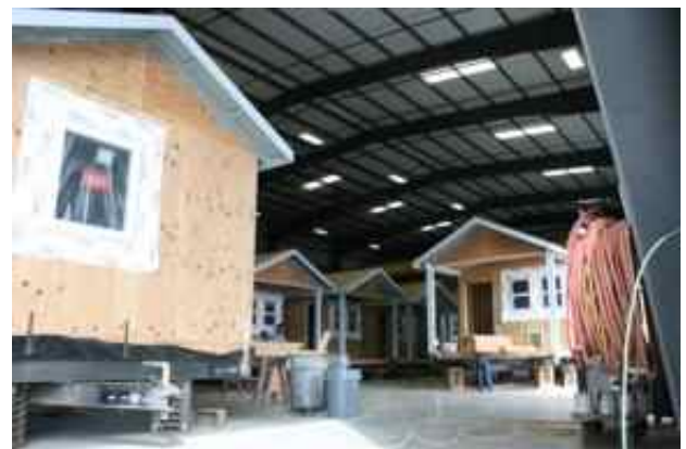
(Above and below) API's self-contained cabin units are energy efficient and constructed indoors and out of the elements, making the assembly units dry and resistant to future mold. These units were ordered by the County of Santa Barbara to be used as revenue producing cabins in recreational areas.
