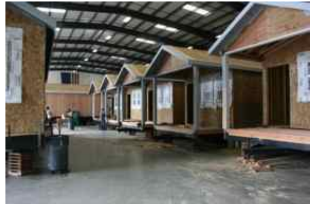
(Above and below) API's self-contained cabin units are energy efficient and constructed indoors and out of the elements, making the assembly units dry and resistant to future mold. These units were ordered by the County of Santa Barbara to be used as revenue producing cabins in recreational areas.
